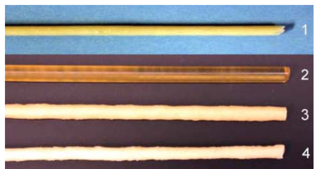
Fig. 1 Compounded rods of the first and second compounding trial. 1: 1CO PLGA 80/20 + DS 8 wt-% ( \text{Ø} \sim 3 mm), 2: 2CO PLGA 80/20 ( \text{Ø} \sim 6 mm), 3: 2CO PLGA 80/20 + DS 4 wt% ( \text{Ø} \sim 6 mm), 4: 2CO PLGA 80/20 + DS 2wt-% ( \text{Ø} \sim 6 mm)
